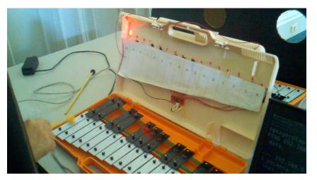
**Figure 4.** Xylophone lighting up the lower G note on the upper display, mallet striking the corresponding aluminum key
